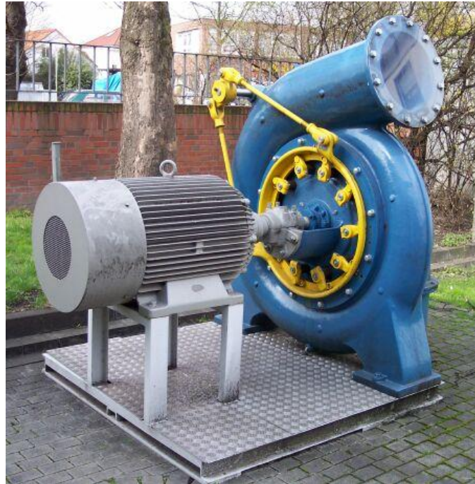
Figure 2-1: Francis Turbine with Generator
